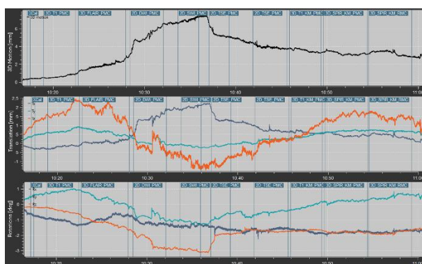
Fig. 2: Plots of rotational and translational motion in three degrees of freedom each, occurring during one complete scan session.
