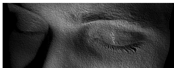
Fig. 1: 3D point cloud of a patient face consisting of thousands of single points.
